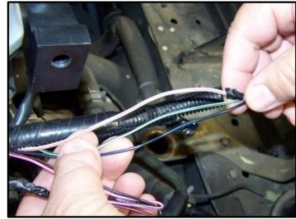
Figure 6: Three MAF wires
