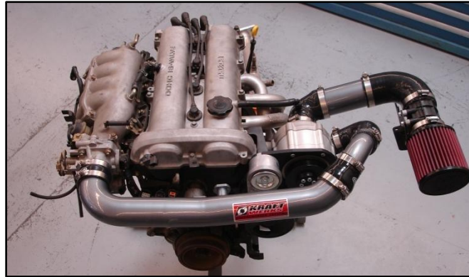
Figure 30: Crossover Tube Installed
