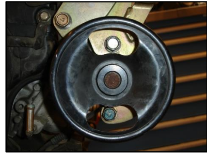
Figure 3: 14mm bolts at 12 o'clock and 6 o'clock
