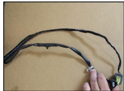
Figure 7: New MAF and IAT wiring harness
